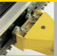
The advanced technology used to build the pulling towers ensures perfect sliding, even after years of work. The pulling towers do not ever have to be removed or dismounted. They slide freely all around the bench and can be blocked at 60 mm intervals. The pulling power remains constant at all heights, the chain always working in a horizontal position.
