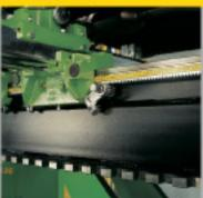
This unique Globaljig solution lets you move any vehicle already on the jig with a simple wrench. The EZ CROSSBEAM can be used on all crossbeams.
