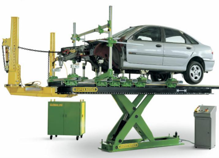
All flanges contain two spring rollers that prevent any lateral movement of the crossbeams. This ensures that the centerline of the bench is always maintained.
