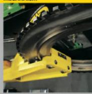
pulling tower has been patented because it ensures easy sliding, not only along the sides but, above all, around curves where it is always perpendicular to the bench.
